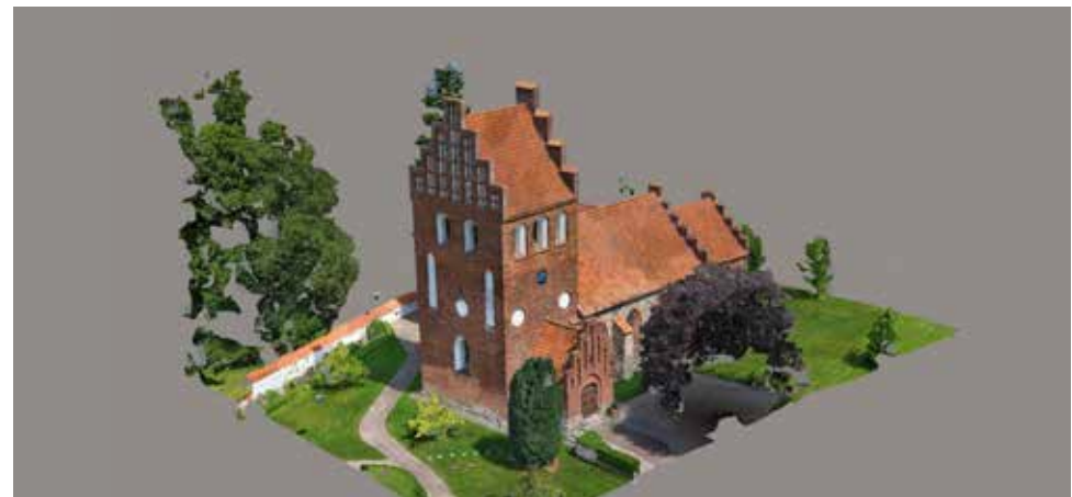
Esbønderup church in 3D, seen here as a "reality twin". It is a photorealistic 3D mesh, made with an AI drone Skydio S2+
