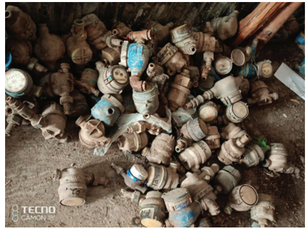
Old and non-functioning water meters collected from customers
